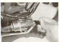
As shown in the right illustration, connect the battery to the fuel pump and measure the pump discharge amount per minute using kerosene.
