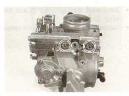
· Remove the throtlle stop screw bracket.
