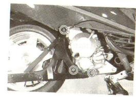
Remove the rear axle nut and take out the rear wheel.
