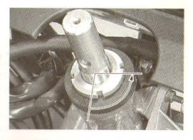
· Fit the washer ① with its tab A engaged with the steering stem groove.
