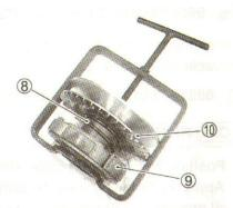
Slowly turn the special tool handle to tighten and align the flats
