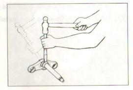
· Drive out the steering stem bearing outer races using the special tools 1 and 2.
