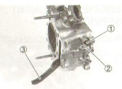
· Compress the valve spring 4 using the special tool.
