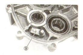
· Remove the oil seal 1 using the special tool.
