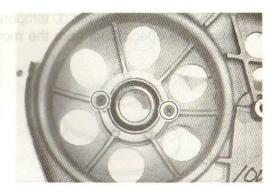
Remove the bearing ① using the special tool.
