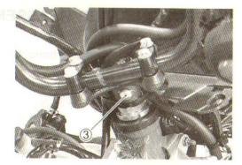
Remove the lock nut 4, washer 5 and steering stem nut 6 and draw out the steering stem.
