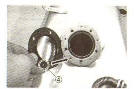
· Tighten the fuel level gauge bolts diagonally and evenly.
