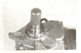
· Install the bearing retainer 2.
