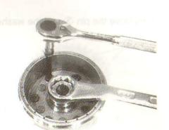
Remove the starter clutch guide ① and starter clutch ② from the generator rotor.
