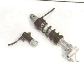
Check the bushing for play and damage. Check the rear shock absorber spring for crack or other damage.
