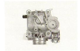
• Remove the float chamber 2 and needle valve 3.
