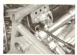
• Remove the engine mounting nut ①, and take out the engine mounting shaft.
