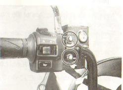
• Remove the brake light switch 1 and brake lever 2.
