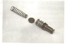
Reassemble the master cylinder in the reverse order of disassembly procedures and observe the following points.
