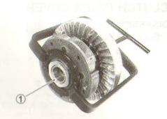
Hold the clutch shoe with the special tool ② and tighten the nut with the special tool ① to the specified torque.
