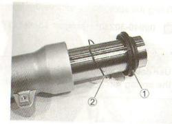
Pull out the inner tube from the outer tube.
