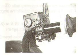
Remove the brake light switch ① and brake lever ②.
