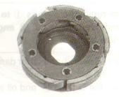
Measure the thickness of clutch shoe at the center position. If the thickness is smaller than the service limit, replace the shoe assembly with a new one.
