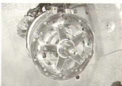
· Loosen the bolt and disassemble the brake disc.
