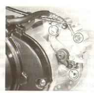
Remove the bolts and take out the brake lock housing 1.
