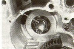
• When installing the balancer driven gear 2, align the punch mark (A) on the balancer drive gear with the punch mark (B) on the balancer driven gear.
