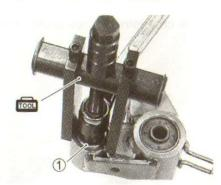
· Press in the bearing using the special tool.
