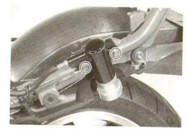
Install the rear suspension on the chassis and tighten with bolts and nuts referring to the illustration in the previous page.
