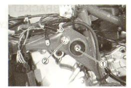
· With the crankcase bracket shaft removal, take out the crankcase bracket 3 and the spacer 4.
