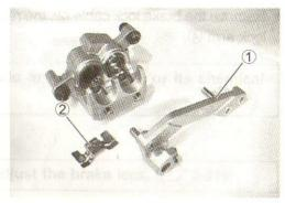
Using an air blow gun, pressurize the caliper fluid chamber to push out the front side piston.
